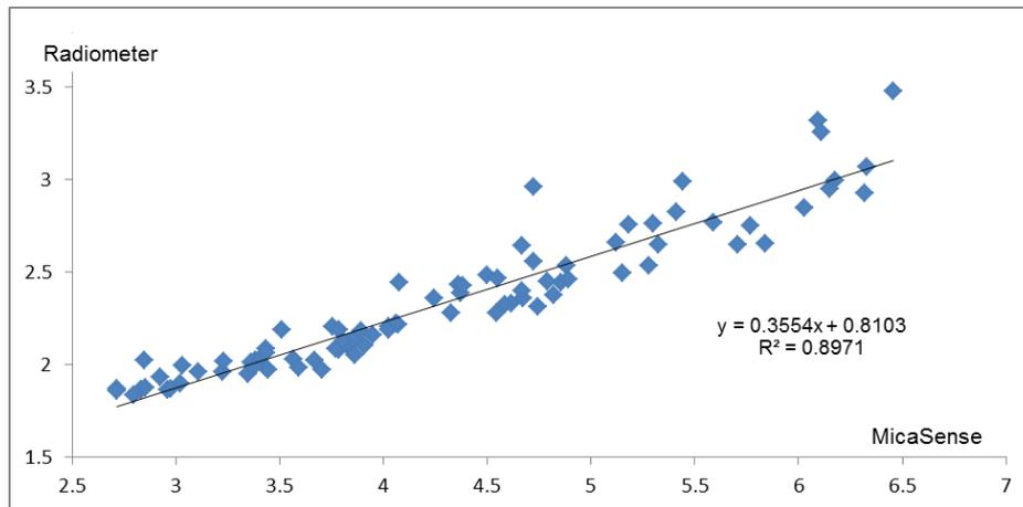
Figure 2. Scatter chart comparing two data set of Vogelmann's Red Edge vegetation index from different sensors measuring the same plots of the wheat field trial at Brookton in August 2015. Ground measurements by an ASD field spectrometer compared with an UAV fly-over carrying a MicaSense RedEdge multispectral camera.
