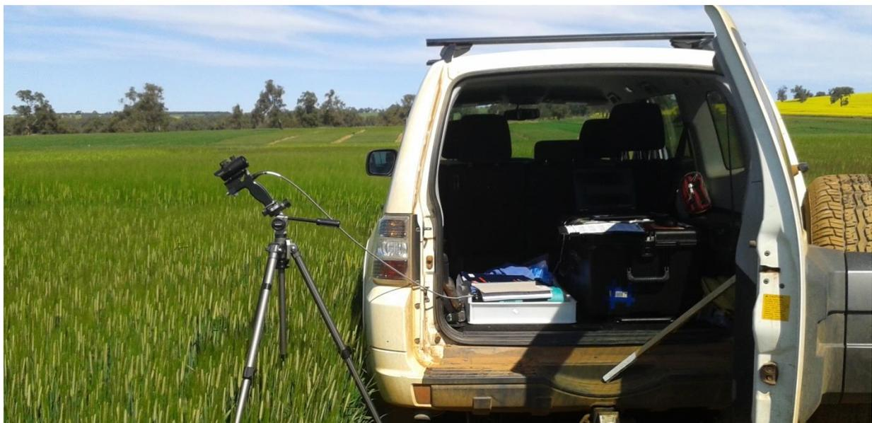
Figure 3 . Setup of the ASD non-imaging radiometer for field measurements in barley at York field site, 2015 .
